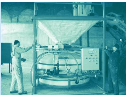
*A recent innovation involves the mixing of salt with water to create a salt brine solution that is applied to roads either as a liquid or mixed with granular salt.*
